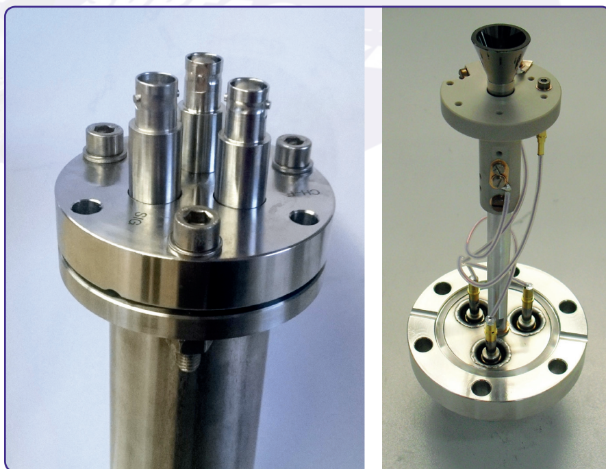
Figure 1: A CEM assembly mounted to the transport container and after removal.
